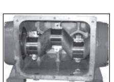
12) Push connecting rod halves together with the crosshead as far as possible into the crosshead guide. Take out bearing cover (14/14A) and push out crankshaft taking particular care that the con rod doesn't get bent. Check surfaces on the connecting rods (24), crankshaft (22) and crossheads (25). Check the surfaces of the crosshead guides in the crankcase for any unevenness.
